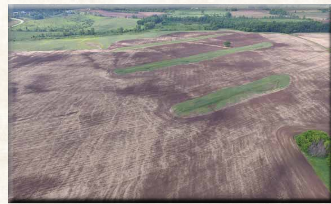
Photo by Jeff Smudde Giant Water and Sediment Control Basins (WASCOBs) were installed in one field in a way that increases efficiency for the farmer and prevents runoff to the stream.
